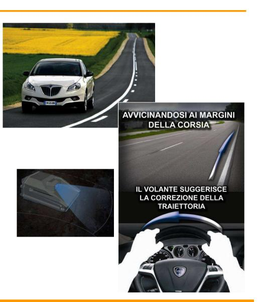
LDW decreases/mitigates lateral incidents, near-crashes, and accidents LDW influences lateral driving performance LDW increases the use of turn indicators in lane change situations LDW increases usage more and more over time LDW increases night driving LDW warning leads to an appropriate driver reaction LDW is well accepted by the driver LDW acceptance/adoption increases with LDW usage
