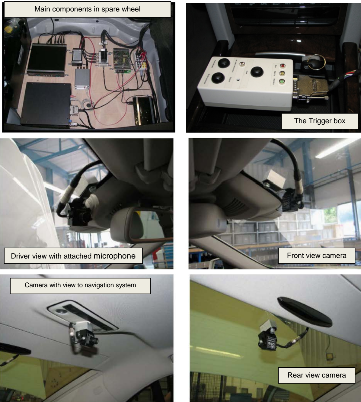
Figure 15: Placement of DAS in a Daimler vehicle.
