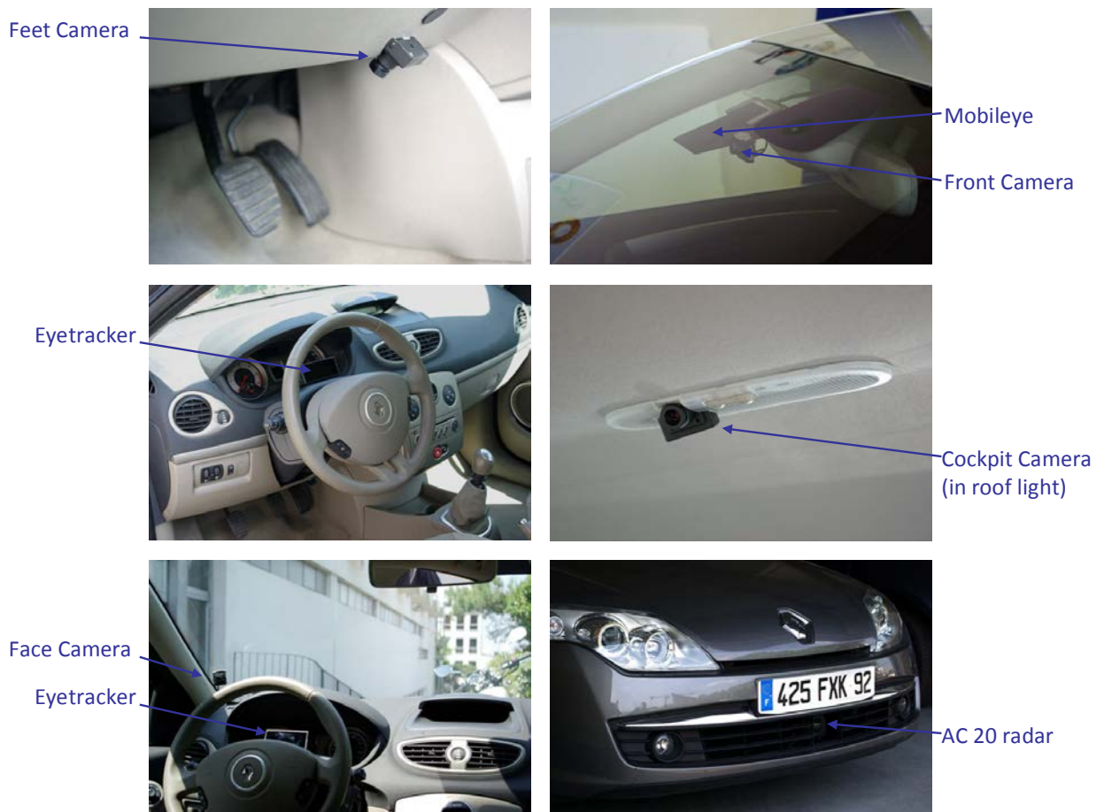
Figure 12: French VMC - Placement of extra sensors and cameras.
