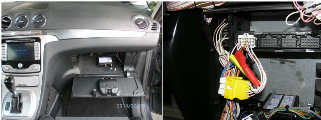
Figure 10: German-1 VMC - Placement of DAS inside glove compartment (Ford) and inside truck cabin (MAN).
